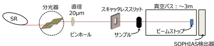
Figure 1. Schematic view of experimental setup.
