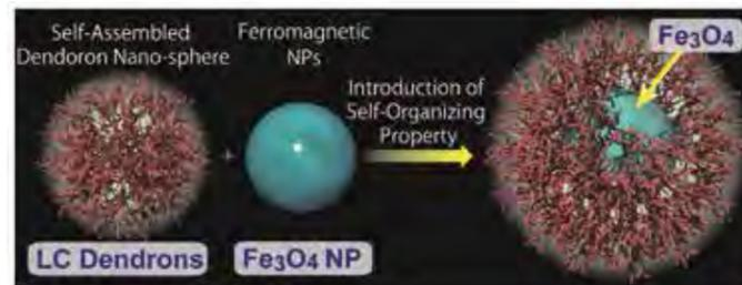
Figure 1. A schematic illustration to obtain organic-inorganic hybrid dendrimer with a  $\text{Fe}_3\text{O}_4$  magnetic NP core.
