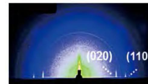
Figure 3. GI-WAXD of a 5 nm-thick PHB film measured with angle of incidence =  $1.3\theta_c$ .
