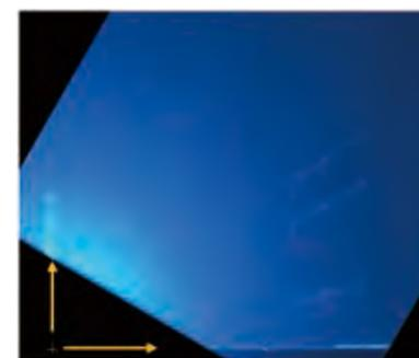
Figure 1. GIWAXS image of spin-coated C<sub>8</sub>-BTBT-C<sub>8</sub> thin film. Cross mark shows specular beam center. Vertical and horizontal arrows correspond to out-of-plane and in-plane direction.
