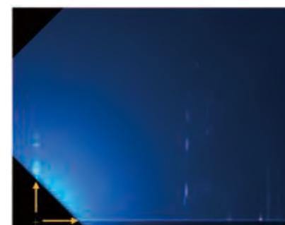
Figure 3. GIWAXS 2D image of bar-coated C<sub>8</sub>-BTBT-C<sub>8</sub> thin film after drying process (before anneal).
