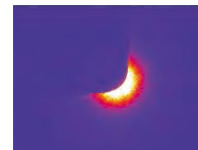
Figure 1. Speckle pattern of silicone resin filled with 10 wt% alumina particles.
