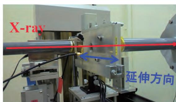
Figure 1. Instrumental setup for SAXS/WAXD measurements at BL03XU.
