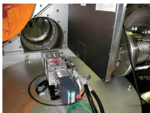
Figure 1. The automatic bar-coating machine for time-resolved GI-SAXS/WAXS was set on the experimental hutch I of BL03XU.
