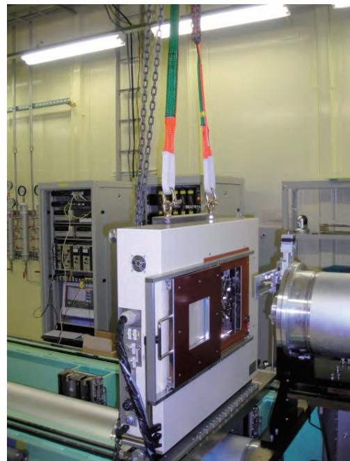
Figure 1. Picture of biaxial stretching machine set on the BL03XU beamline at SPring-8.
