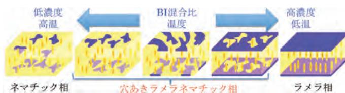
Figure 1. Schematic images of structures of the perforated lamellar phase.
