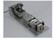
Figure 1. A miniature axial compression testing machine used for experiments.
