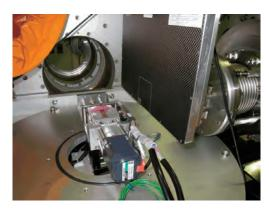
Figure 1. The automatic bar-coating machine for timeresolved GI-SAXS/WAXS was set on the experimental hutch I of BL03XU.
