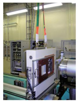
Figure 1. Picture of biaxial stretching machine set on the BL03XU beamline at SPring-8.
